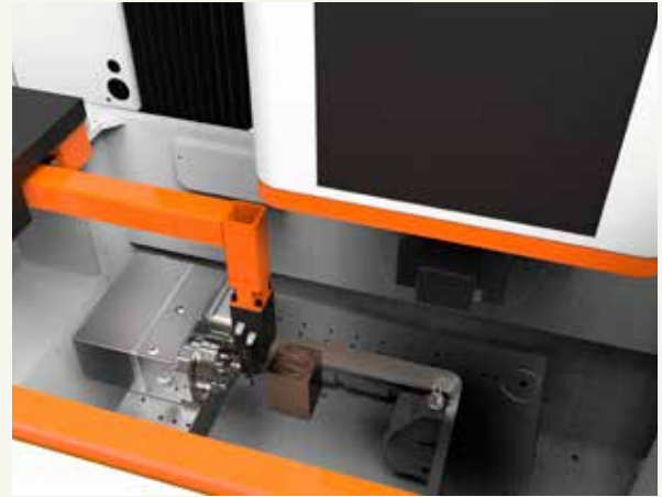
WorkPal 1 Application example: B-axis for Wire-cutting EDM (wire EDM).
