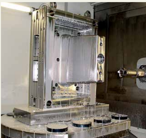
System 3R Delphin - the modular clamping system
