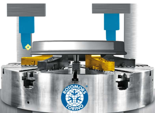
Second operation: the clamping is performed on the surface machined in the first phase through the second set of 3 down-clamping jaws
